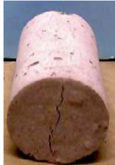
Fig. 10. Cylindrical sample after a splitting test displaying diametrical plane crack, right failure.
